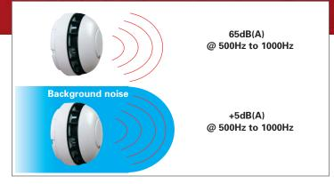
The minimum sound level of a sounder device should be 65dB(A) or 5dB(A) above a background noise which is louder than 60dB(A) (if lasting more than 30 seconds) and at a frequency of between 500Hz and 1000Hz. The maximum sound level should not be greater than 120dB(A) at any normally accessible point. May be reduced to 60dB(A) in stairways, enclosures up to 60m<sup>2</sup> and specific points of limited extent.
