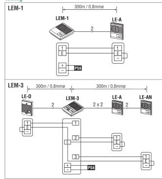
★ Do not remove shorting link on subs. PS6: PS-0603DIN
